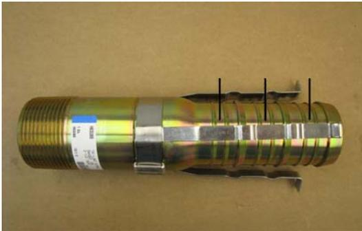
1. Identify the location where clamps should be installed which is between sealing bars once the hose has been properly placed. Sealing bars are less prominent than holding bars.
