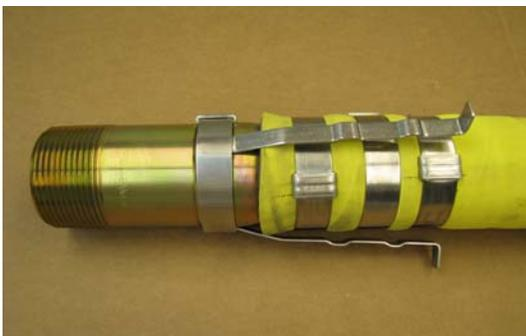
3. Position and install a clamp under the Tie strips directly over each mark on the hose. The location of the clamp's buckle should be 120° - 180° from each other.
