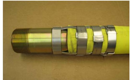
4. Position and install a clamp over the Tie-strips. This secures the hose to the Tri-Lokt hose nipple and help prevents slippage.
