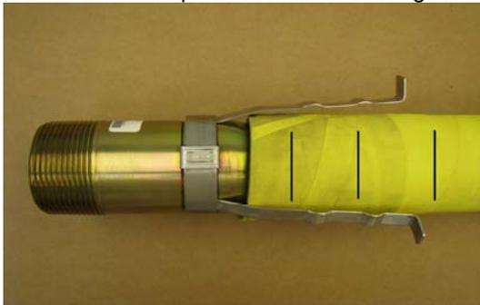
2. Mark the hose as shown; this will help locate the proper placement of clamps.
