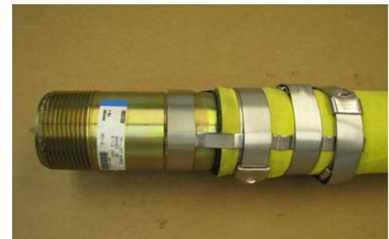
5. Apply a clamp over the ends of the Tie-strips for additional lock.
